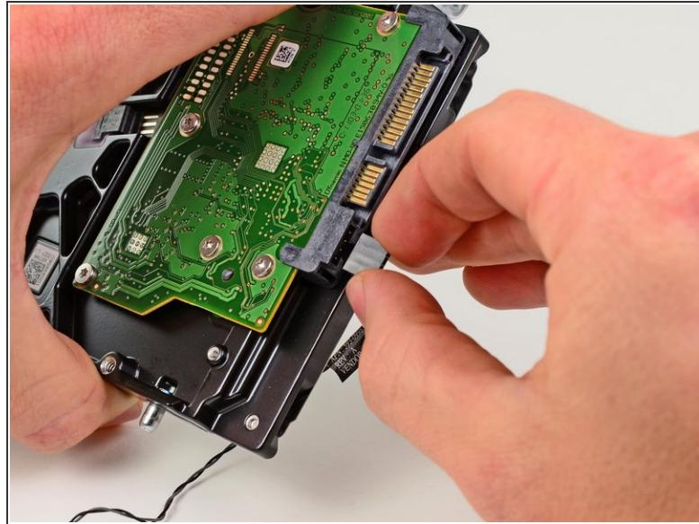
**⚠** Before disconnecting the thermal sensor cable, take note of its orientation. It is extremely important to reinstall the connector in the current orientation so the fans will not run at full speed. If you have multiple pins on your replacement hard drive, put the connector closest to the SATA connections and closest to the PCB board.
